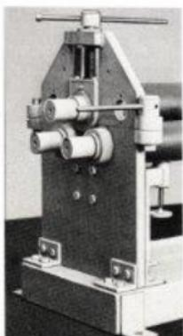
SPECIFICATIONS – CONVENTIONAL PYRAMID TYPE PLATE CURVING ROLLS TO 12MM (½") CAPACITY
